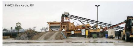
At peak, RCP Block has used the equivalent of 300 yd./day of recycled aggregate. The company utilizes an impact crusher mill at its Otay Mesa, Calif., plant (shown here) near the Mexico border, and a jaw roller crusher at a Santee, Calif., operation. Based in Lemon Grove, Calif. (headquarters office, above), RCP is no stranger to aggregate production, as it operates a sand pit in Santee to supply some of its fine aggregate requirements for both plants.
