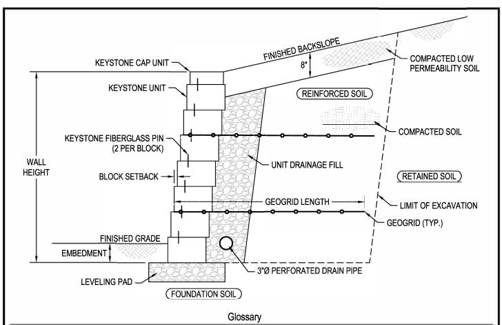
KEYSTONE UNIT - Keystone Compac III pinned units. Fill core with 3/4" clean crushed stone.
